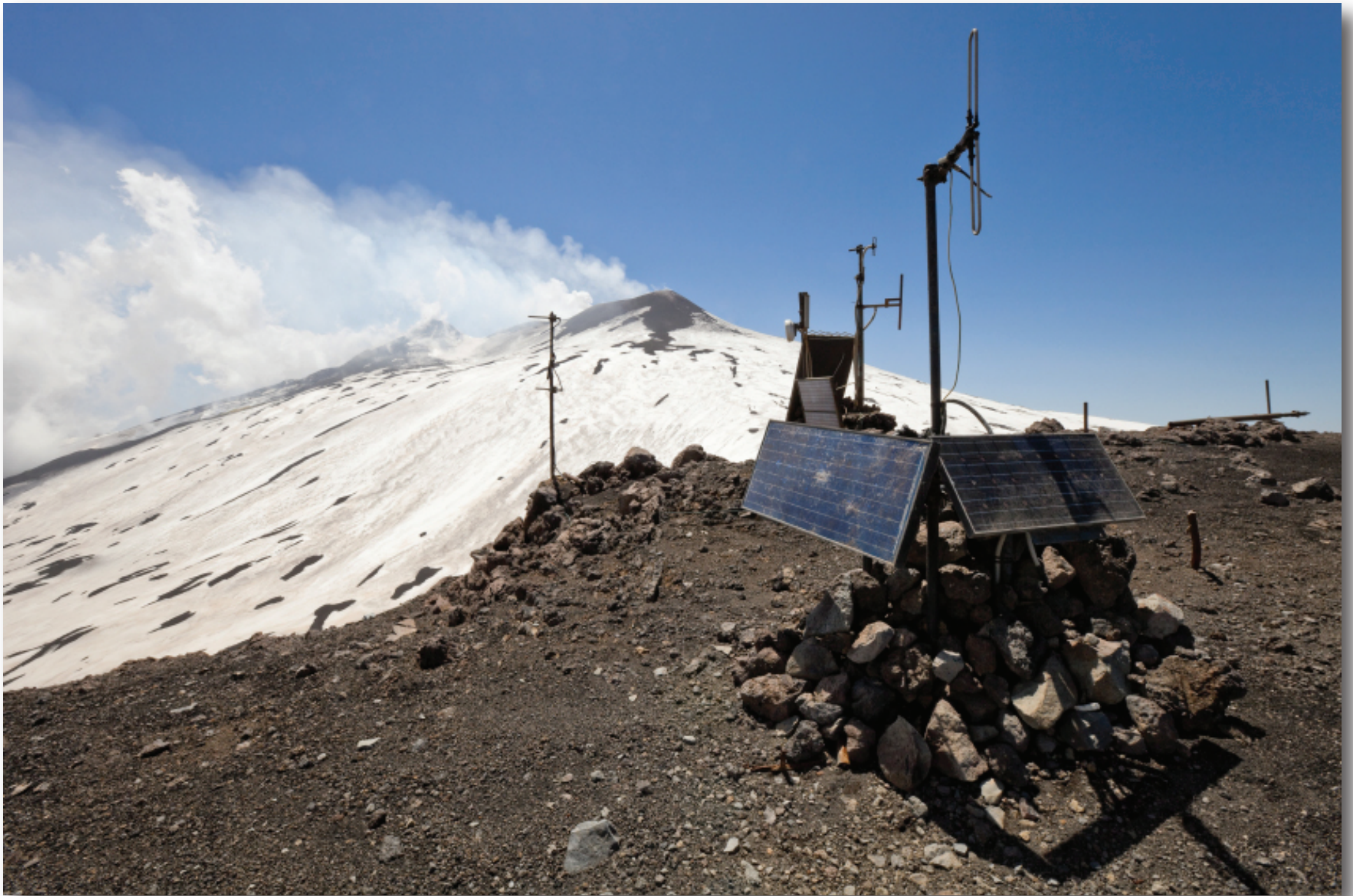
Volcanic Action is monitored by scientific equipment that picks up vibrations in the Earth's crust.
