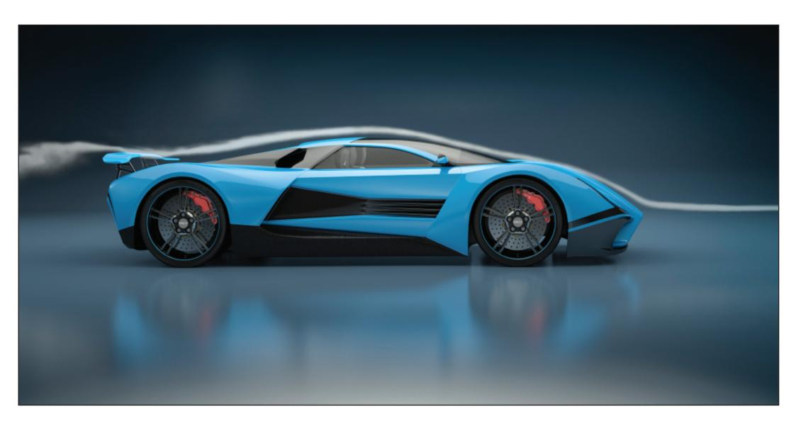
Designers use curved lines in their designs to encourage air to flow quickly over the top of a form. They can test the streamlining of a car by placing it in a wind tunnel. A thin line of smoke is released in front of the car to demonstrate the flow of air over the design model.
